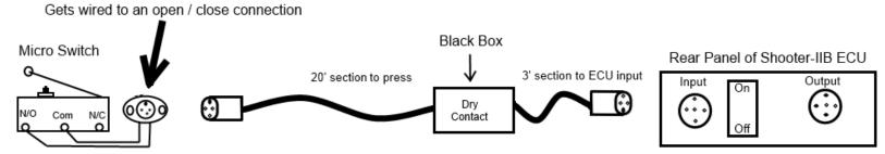
The "Dry Contact" Connection would be wired to a new or existing Micro Switch or any connection such as a relay with a open / close per sheet count no voltage connection.
