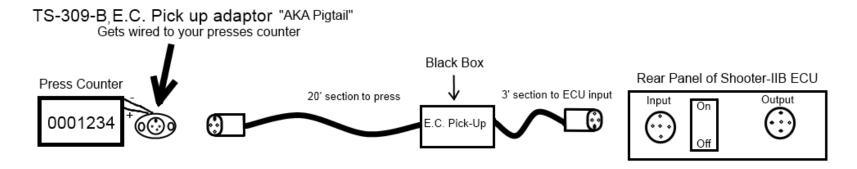
The E.C. Pick up adaptor would be wired in to the the Presses Counter or Count pulse. This is a 2 wire connection that requires a high / low voltage pulse from 8V - 120V AC or DC per printed sheet.
